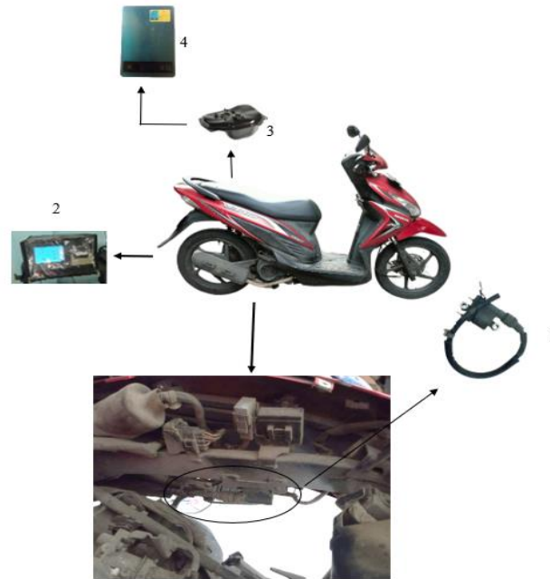
Figure 1. Schematic of testing equipment. 1. Honda Vario 110 FI, 2. Gas analyzer, 3. Fuel tank, 4. Digital scale, 5. Ignition coil.
