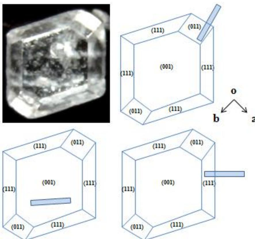
Figure 6. Schematic heterogeneous nucleation of  $\beta$ -form possibly occurred on the different surfaces of  $\alpha$ -form crystal
