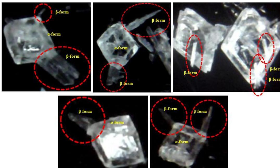
Figure 5. Heterogeneous nucleation of  $\beta$ -form occurred on surface of  $\alpha$ -form crystal
