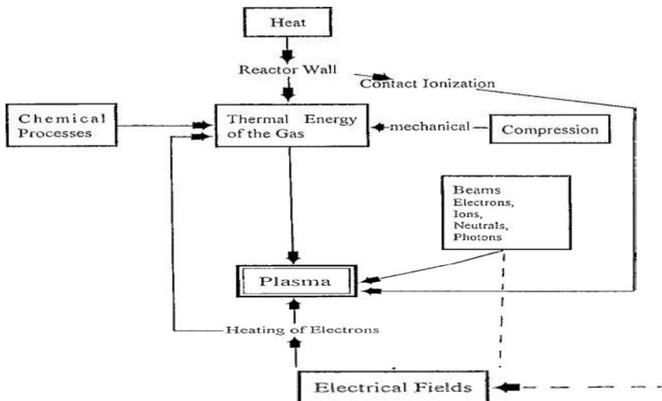
Figure: Various ways of supplying the necessary energy for plasma generation
