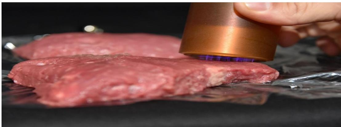
Figure: A plasma torch applied to uncooked chicken
