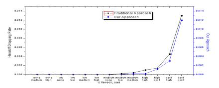
The above fig gives the effect of offered load on handoff dropping rate. In the above fig the proposed method gives best result than the traditional approach even offered load varies. Our proposed model reduces the hand off dropping rate by up to 0.480%.
