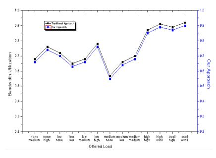
In the above fig, our proposed approach shows better result than the traditional approach on overall bandwidth utilization even if offered load varies. In the above graph we considered bandwidth utilization on y axis and load on x axis. This proposed method increases bandwidth utilization by 2.5% as compared with traditional approach.
