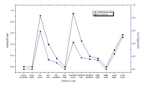
The above fig shows the result over the handoff rate and offered load. The handoff ratio is defined as the ratio of the total number of handoff execution to handoff decision. In the above simulation we considered the number of handoff decision are similar in the both traditional and our approach. In proposed approach the handoff rate is always smaller than traditional approach.
