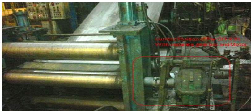
Fig. Pay-OFF4HI with separate Gear box and Motor
