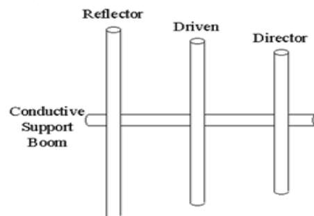
Figure 1.1 Element Yagi-Uda Antenna
