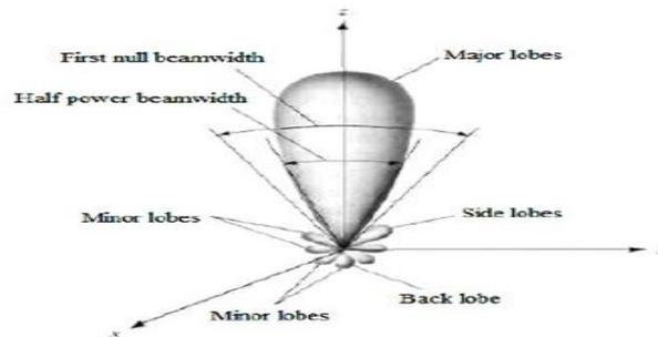
Figure 2.1 Parts Of Radiation Pattern
