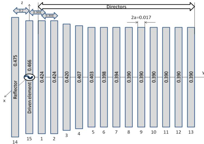
Figure 6.1 NBS Parameters for Yagi-Uda Antenna
