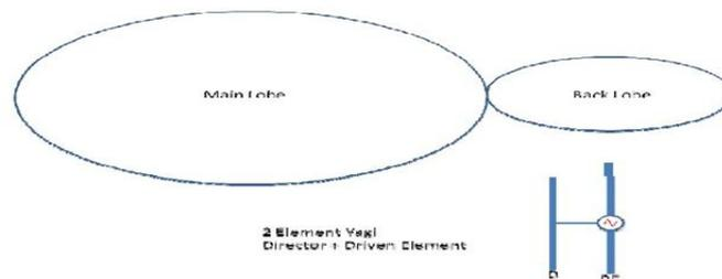
Figure 3.2 Element Yagi (Director+Driven Element)
