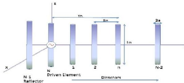
Figure 4.1 Yagi-Uda Antenna's Set Up
