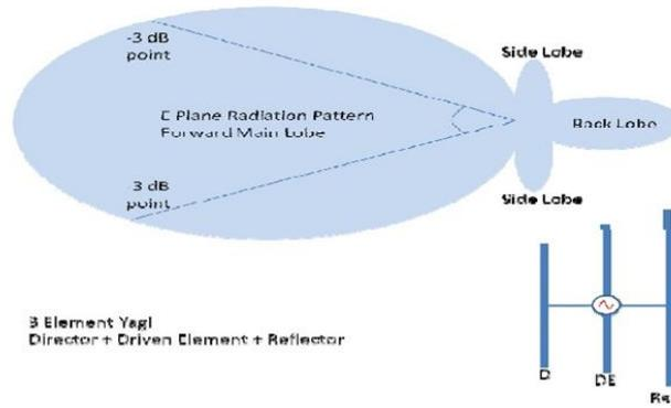
Figure 3.3 Element Yagi (Reflector+Driven Element+Director)
