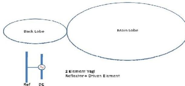
Figure 3.1 Element Yagi (Reflector+Driven Element)
