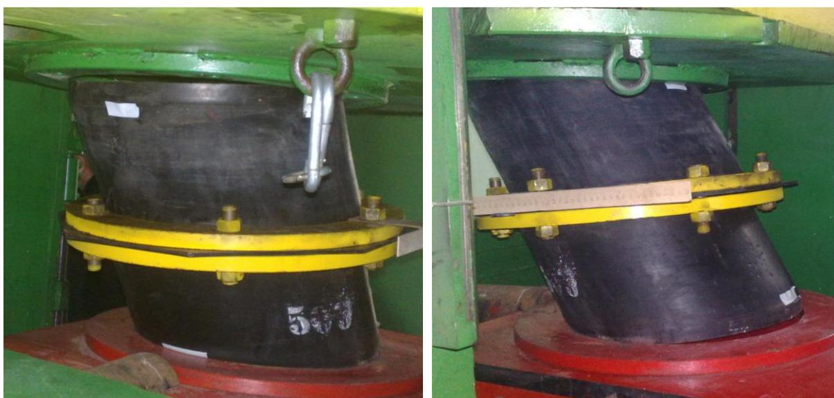
Figure 4. Moment of testing at the "Firm TNT" LLC of the node with seismic isolators installed on top of each other under the action of horizontal force at the level of the lower plate (red color) of the lower seismic isolator
