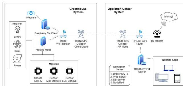
Figure 6: Greenhouse System and Operation Center System
