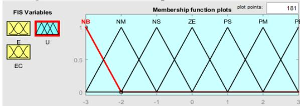
Figure 6. The membership functions of the power supply U
