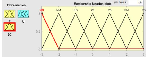
Figure 5. The membership functions of error EC
