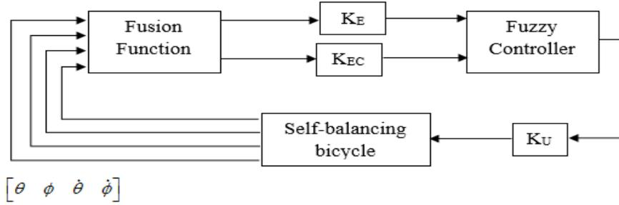
Figure 3. The model of fuzzy-LQR controller
