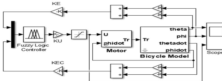
Figure 7. The scheme of Fuzzy-LQR controller
