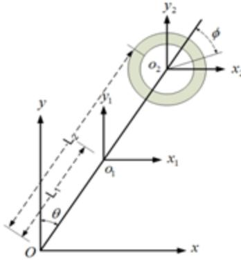
**Figure 1.** The model of self-balancing bicycle using reaction wheel [11]
