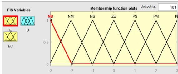
Figure 4. The membership functions of error E
