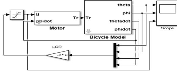
Figure 2. The scheme of LQR controller
