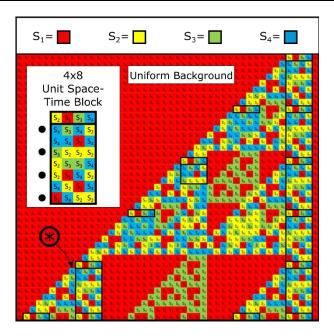
The corresponding space-time crystal generated from the counter-clockwise cyclic rules is shown with the same initial configuration as in Fig. 3. This crystal differs from Fig. 3 on every other row as indicated by the black dot. Half of the data or the computing generated from the two cyclic rules is wasted because they are not useful to the generation of the space-time crystal in nature.
