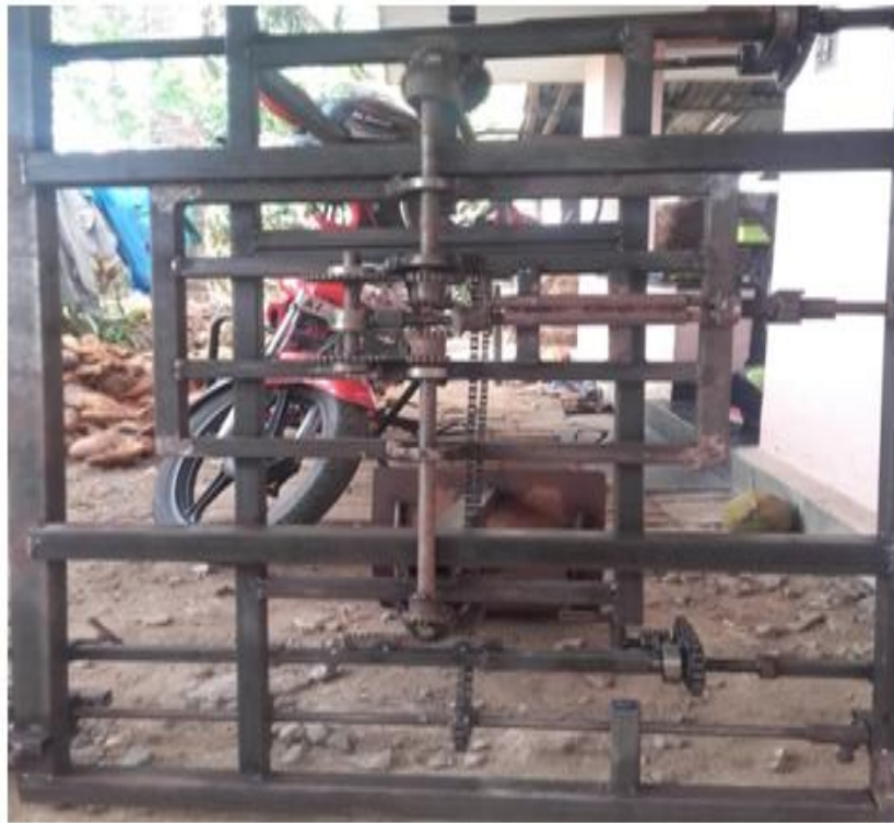
Fig.4.2. Mechanism of four wheel steering system
