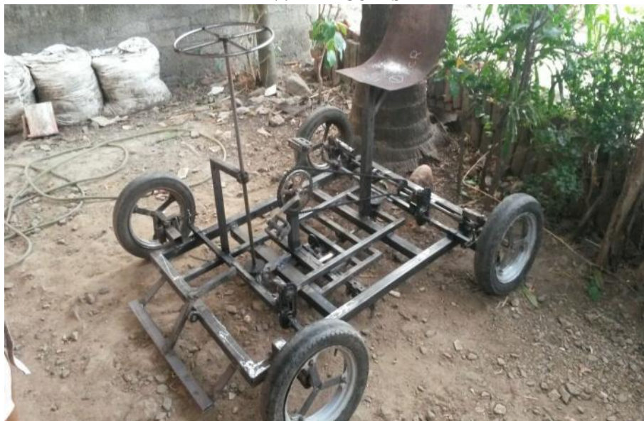
Fig.4.1.Manufactured model of four wheel steering system.
