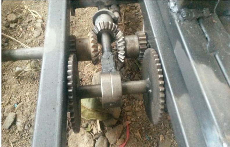
Fig.3.1. Working of Four Modes of Steering Mechanism
