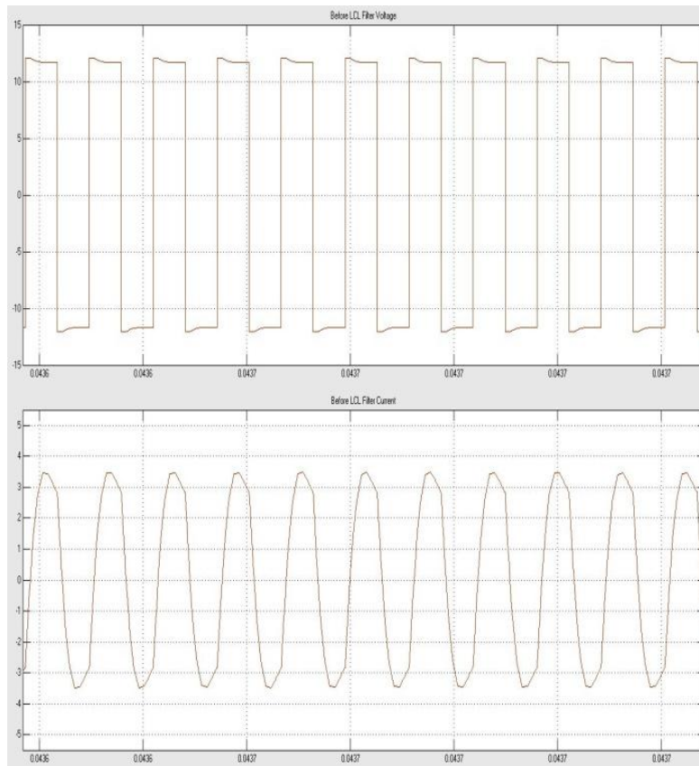
Figure6: Input voltage & current for the Double LCL filter
