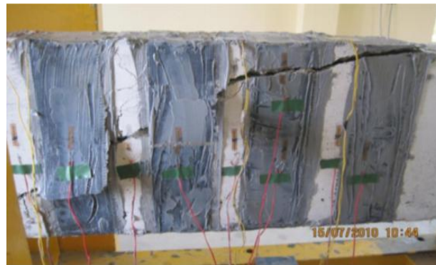
Fig. 4: Cracking and failure pattern of beam C2.5-UA-S
