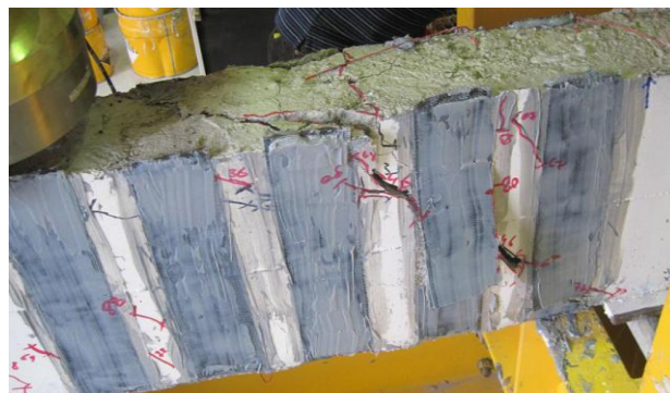
Fig. 5: Cracking and failure pattern of beam C2.5-U-S
