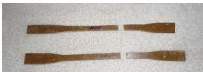
Fig 2: Tensile Test Specimen After Test
