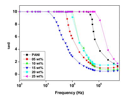
Figure 5 shows the variation of tan  $\square$  as a function of frequency of PANE V<sub>2</sub>O<sub>5</sub> composites at different weight percentage
