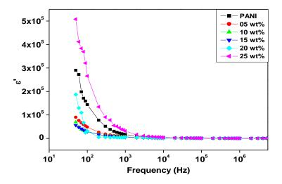
Figure 4 shows the real part permittivity as a function of frequency of PANI- V<sub>2</sub>O<sub>5</sub> composites at different weight percentage
