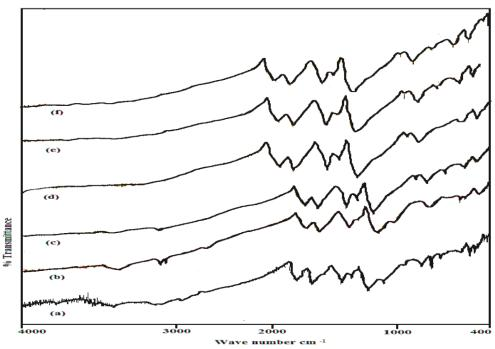
Figure 1(a-f) shows the FTIR spectra of PANI/V<sub>2</sub>O<sub>5</sub> composites of different weight percentage.
