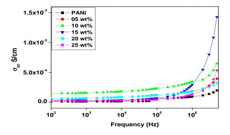
Figure 3 shows the variation of  $\Box_{ac}$  conductivity as a function of frequency for polyaniline –  $V_2O_5$  composites (different wt %).
