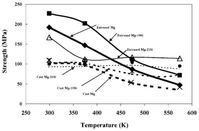
Fig 1: The tensile strength of the extruded and cast Mg-Si alloys [15]
