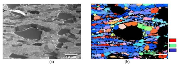
Fig 6: Microstructure of SiC particle reinforced 2080 Al matrix composite after hot extrusion.
