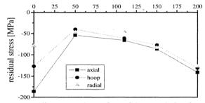
distance to the surface of the sample  $[\mu m]$ Fig 9: Residual stress in Si-particles, at 450°C [13]
