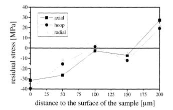
Fig 10: Residual stress in Al- matrix at 400°C [13]
