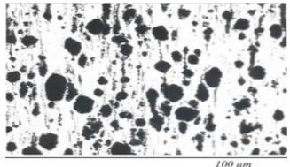
Fig 5: Microstructure of extruded 7475 Al -25 vol.% Al<sub>2</sub>O<sub>3</sub> particles(40 µm) [14]
