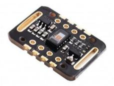
MAX30102 is a combination of pulse oximeter and heart rate monitor biosensor module. It combines red LED a nd infrared LED, photodetectors, optical components, and lownoise electronic circuitry that suppresses ambient light. Devices worn on the fingers, ears and wrists to monitor h eart rate and heart rate collect oxygen in the blood.
