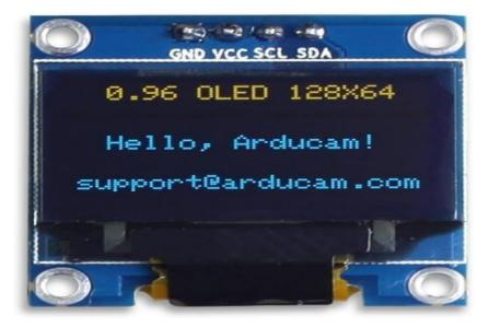
The 0.96 inch OLED Display Module - SPI/I2C - 128×64 - 7 Pin (Blue) are one of the most attractive displays available for a microcontroller.
