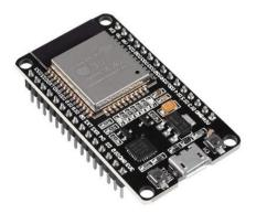
The ESP32 is integrated with onboard antennas, RF baluns, power amplifiers, low-noise receiver amplifiers, filters and power control modules. ESP32 adds invaluable functionality and versatility to your application with printed circuit board (PCB) codes.
