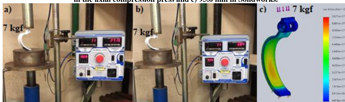
Figure 20. Application of 7 kgf in ABS material with a displacement of a) 27.15 mm, b) 45.7 mm in the axial compression press and c) 93.6 mm in Solidworks.
