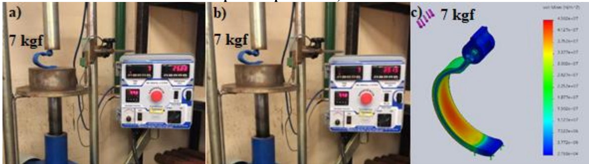
Figure 17. Application of 7 kgf in PETG material with a displacement of a) 25.88 mm, b) 78.87 mm in the axial compression press and c) 48.96 mm in Solidworks.
