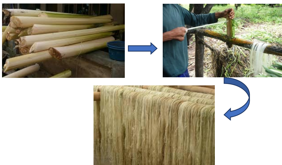
Figure2. The Musa acuminata stem fiber (MASF) extracted process
