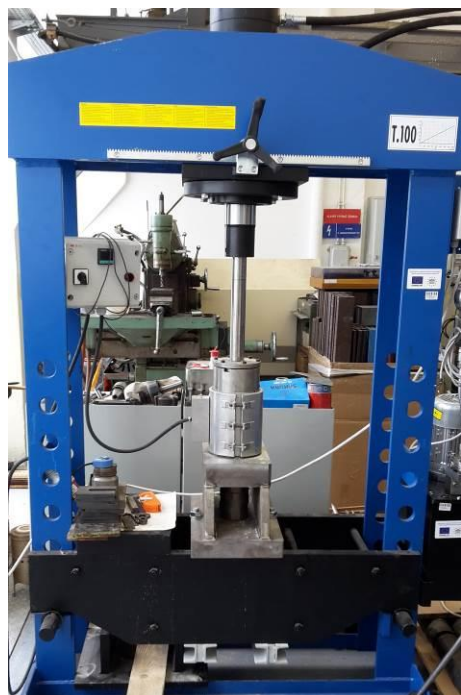
Figure 5 Pressing equipment in a hydraulic press
